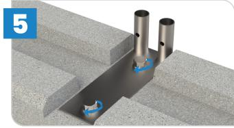
Secure the connecting bracket in place using high tensile bolts.
