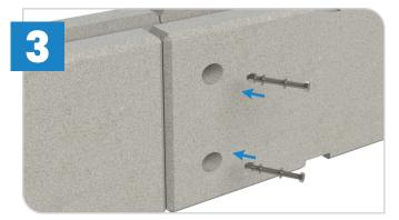
Insert high M24 high-tensile bolts into the holes at the end of the barrier to fix in place. The barriers can also be fixed to the carriageway if required. Simply bolt the anchor plates on the underside of the barriers to the ground.
