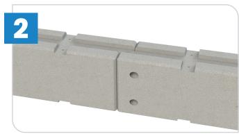
Place the barriers close to each other so that they interlock. The ends of these barriers feature 'scarf' joints, which secured together using high-tensile bolts.
