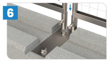
Slot the mesh fence panels into the holes in the connecting bracket and tighten the screws to keep in place.
