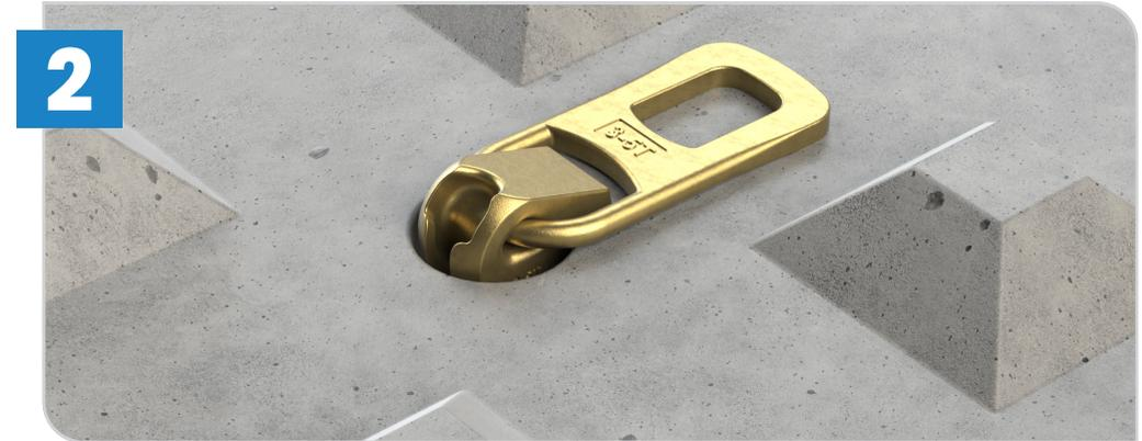
The ring head of the clutch has a locking bolt, which helps safely lock into plate anchors while the concrete panels are in the lifting process.
