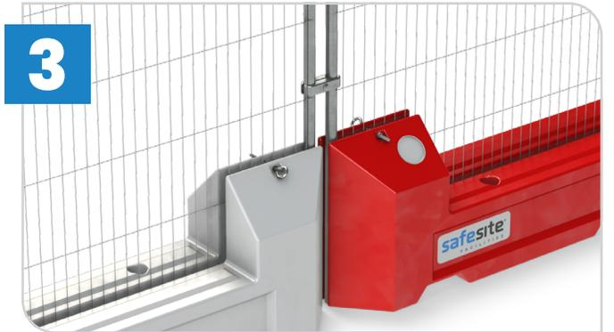
To attach the mesh fence panel, slide the legs of the mesh fence into the slots at either end of the barrier and make sure it's secure.
