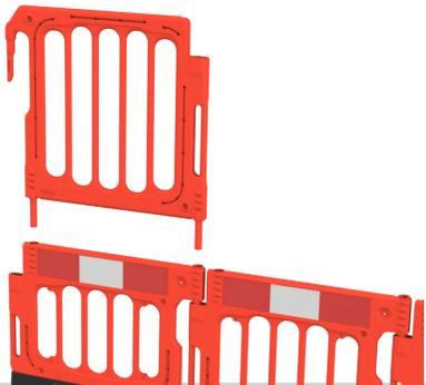
You can increase the overall height of the barrier with an extension. To install the fence extension, line up the bars at the bottom of the fence with the holes on the top of the WonderWall barrier. Slot into place until secure.
